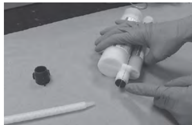
Remove and discard plastic plugs in outlet ports
