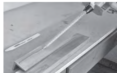
Dispense adhesive through static mix tip on assembly
