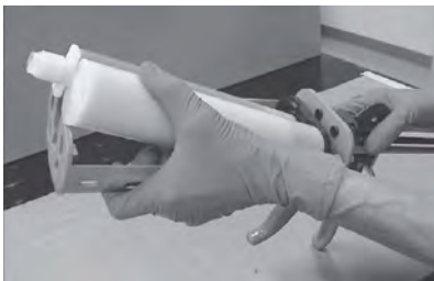
Load cartridge into dispensing gun
