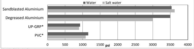
(\*): UP-GRP, PVC, substrate failures observed.
