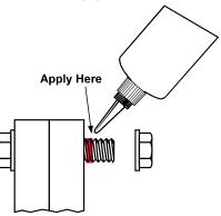
6. **For Blind Holes**, apply several drops down female threads into the bottom of the hole. As threads are engaged, compressed air forces the product upwards into the threads.
