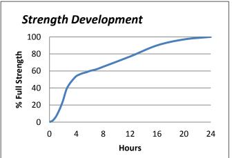
Graph shows typical strength development of bonded components at 23°C. An increase of 8°C in temperature will halve the cure time. Lower temperatures will result in a slower cure time.
