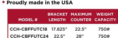
Weight capacity is based on evenly distributed static loads
