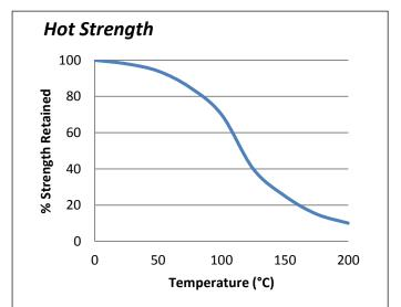
UV683 can withstand higher temperatures for brief periods (such as for paint baking and wave soldering processes) providing the joint is not unduly stressed. The minimum temperature the cured adhesive can be exposed to is -55°C (-67°F) depending on the materials being bonded.
