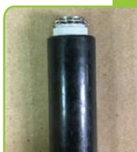
Use compressed air to clear the hole of debris. Use the Go/No Go gauge to test the hole. If the size labeled "No Go" fits, the hole is larger than recommend and the anchor may not perform according to specification. **When manual drilling the hole may be slightly large or out-of-round at the top of the hole. As long as the hole is sized correctly at the bottom, the anchor will perform at or near full strength.**
