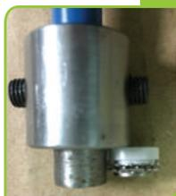
Set the stop collar for the height of the anchor plus 1/16". For most applications including undermount sinks, the 2 crown 6.5mm height anchor (2S) is recommended. For this anchor, set the stop collar for around 5/16 or 8mm from the cutting edge. This extra depth is important as the first 1/16" of drilling depth will be wider or out of round. As the bit drills deeper, the hole typically becomes more accurate.
