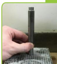
Use the "Go" side of the "Go/No Go" gauge and gently tap the anchor with a mallet until it is fully seated at the bottom of the hole. **The anchor must "bottom out" in the hole to work correctly.** If the anchor is not fully seated, then the post will spin freely and not tighten down once inserted.
