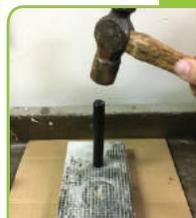
Thread a Keep-nut anchor on the setting tool and gently tap into the hole using a rubber mallet or dead blow hammer.
