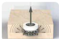
**6** The "no-through" threading of the internal bushing prevents over tightening.
