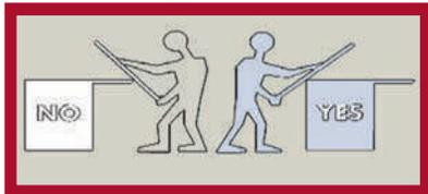
NEVER set tops directly on plate or bracket at an angle when setting tops.
