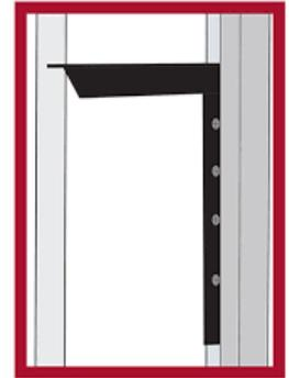
The CounterBalance **Hybrid Bracket** is an easy install to support overhangs on stone and solid surface countertops. These products give your customers alternative to banging their knees on pricey corbels and provide superior support and security. These low-profile brackets are hidden from view offering a clean, modern look.
