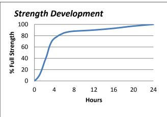
Graph shows typical strength development of bonded components at 23°C. An increase of 8°C in temperature will halve the cure time. Lower temperatures will result in a slower cure time.
