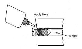
Avoid touching the bottle tip to the metal surface. Not recommended for pre-assembled threads in a blind hole.
