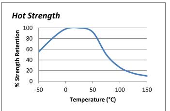
"Hot strength" shear strength tests performed on mild steel. 24hr cure at room temperature and conditioned to pull temperature for 30 minutes before testing.
