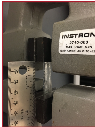
Above, a cured sample of Chem-Set ™ 73 flexible cyanoacrylate is stretched to four times its original length!
