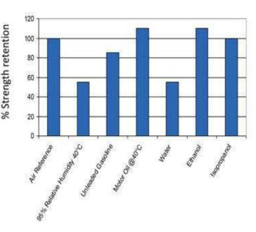
Specimens were immersed for 1000 hours at 22°C (unless otherwise stated)
