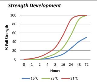
Graph shows typical strength development of bonded components. An increase of 8°C in temperature will halve the cure time. Lower temperatures will result in a slower cure time.
