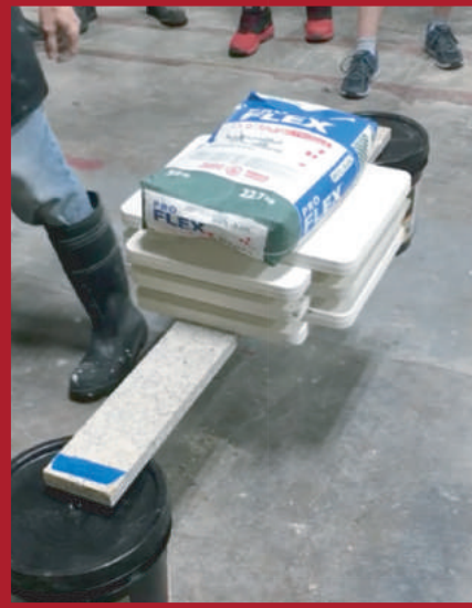
250lbs of weight on 5" x 54" granite rail with no breakage!
