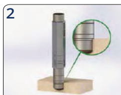
2 Verify hole diameter using Go/No-Go gauge. Check hole depth against reference line on Go side of gauge.
