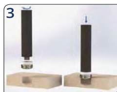
3 To ensure correct installation it is recommended that a threaded mandrel is used. Fully screw on the insert and drive into the hole.
