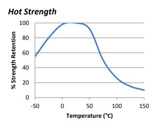
"Hot strength" shear strength tests performed on mild steel. 24hr cure at room temperature and conditioned to pull temperature for 30 minutes before testing.
