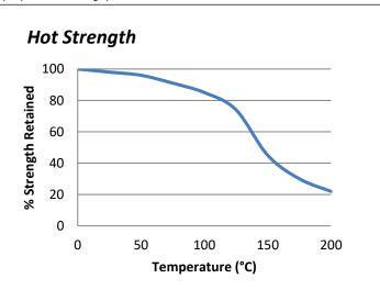
"Hot strength" shear strength tests performed on mild steel. Fully cured then conditioned to pull temperature for 30 minutes before testing. ES550 can withstand higher temperatures for brief periods (such as for paint baking and wave soldering processes) providing the joint is not unduly stressed.
