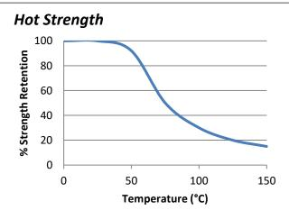
"Hot strength" shear strength tests performed on mild steel. Fully cured specimens conditioned to pull temperature for 30 minutes before testing at temperature. ET515 can withstand higher temperatures for brief periods (such as for paint baking and wave soldering processes) providing the joint is not unduly stressed. The minimum temperature the cured adhesive can be exposed to is -55°C (-65°F) depending on the materials being bonded.
