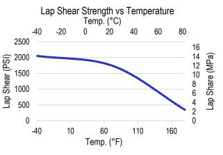
\*Data represents good faith obtained ranges and is not for use for specification purposes. CF - Cohesive failure
