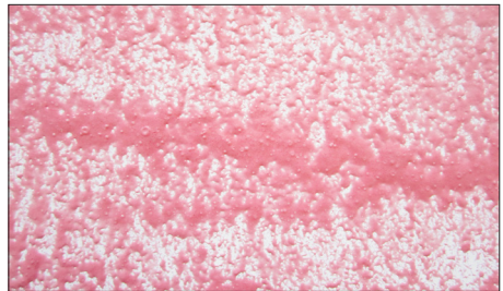
COVERAGE TOO HEAVY
