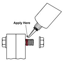
For Blind Holes, apply several drops down the female 6 threads into the bottom of the hole. As threads are engaged, compressed air forces the product upwards into the threads.
