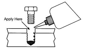
7. Assemble and tighten as usual. When tightening to established torgue values, torgue compensation is not required.
