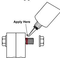
For Blind Holes, apply several drops down the female threads into the bottom of the hole. As threads are engaged, compressed air forces the product upwards into the threads.
