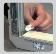
Insert glue-catcher in the rebate of the mitreForma™
