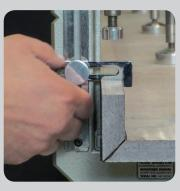
Use the retaining arms to ensure fascia is held firmly against the back guide
