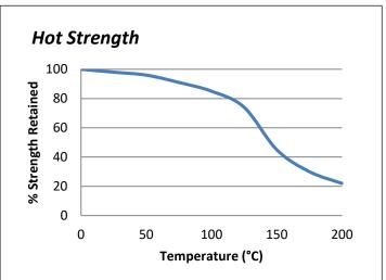
"Hot strength" shear strength tests performed on mild steel. Fully cured then conditioned to pull temperature for 30 minutes before testing. ES562 can withstand higher temperatures for brief periods (such as for paint baking and wave soldering processes) providing the joint is not unduly stressed. The minimum temperature the cured adhesive can be exposed to is -40°C (-40°F) depending on the materials being bonded.
