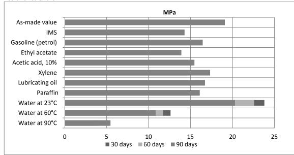
Lap shear strength versus tropical weathering (ISO 4587) (typical average values)
