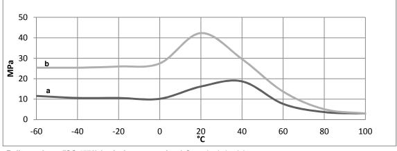
Roller peel test (ISO 4578) (typical average values) On etched aluminium
