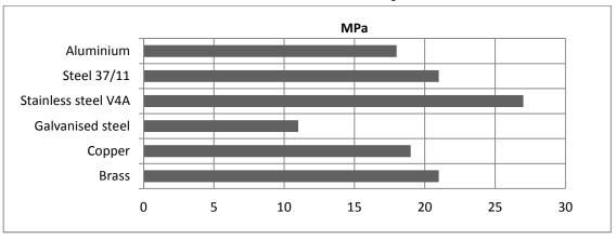
Cured for 16 hours at 40°C and tested at 23°C. Pretreatment - Sand blasting
