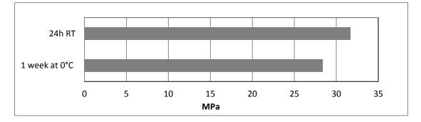
Average lap shear strengths after application, bonding and curing under water (ISO 4587) (typical average values)
