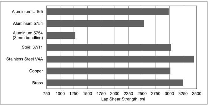
Note: ARALDITE® 2053-15 is not suitable for galvanized steel, for this type of substrate the ARALDITE® 2047-1 or ARALDITE® 2051 can be used.
