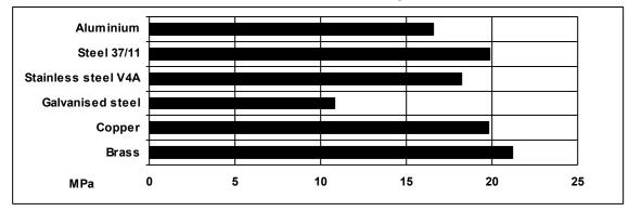
Cured for 16 hours at 40°C and tested at 23°C. Pretreatment - Sand blasting
